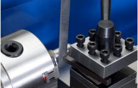
Using the standard tool post, you adjust the tool bit height using shims under the tool bit. You can get an economical set of shims, about the right size, at any auto parts store. Purchase a set of feeler gages and remove the pivot pin.
