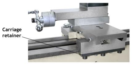
There are several fasteners in the carriage retainers. The socket head cap screws are used to adjust the position of the retainers. The setscrews and lock nuts lock the adjustments in place.
