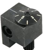
The gear on the threading dial has 16 teeth, and the lead screw has 16 threads per inch, so each revolution of the threading dial represents one inch of
